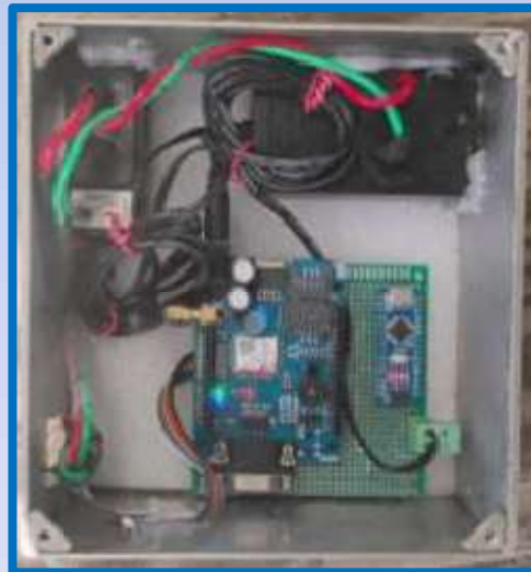
Sensor & wireless data transfer for long life SWA battery
